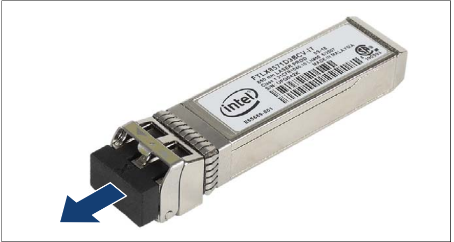
Figure 38: Removing the protective optical port plug
